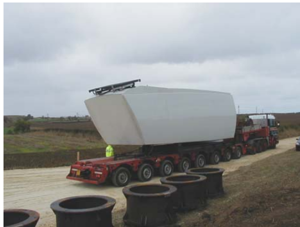
Low loader delivering a nacelle. The nacelle is bolted to the top tower section and contains the gearbox and generator. The blade assembly is bolted onto the end of the nacelle to the right of the picture. The nacelle weighs approximately 88 tonnes.
