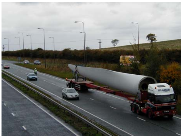
Single turbine blade on extendable trailer with police outrider escort on A19.
