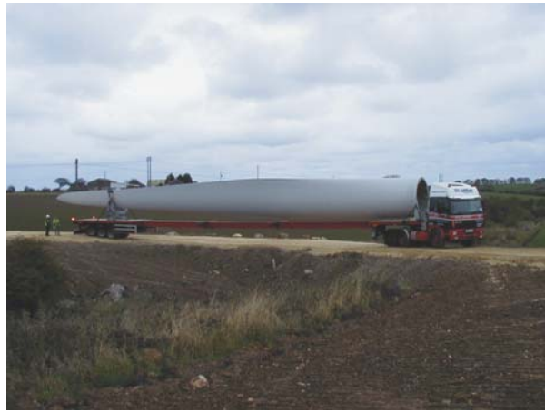
Single blade on site access road. These blades are 38 metres long and weigh approximately 10 tonnes.
