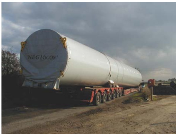
The tower is delivered in 2 sections. The overall length of this vehicle and tower section is approximately 41 metres. The diameter of the base is 4.2 metres.
